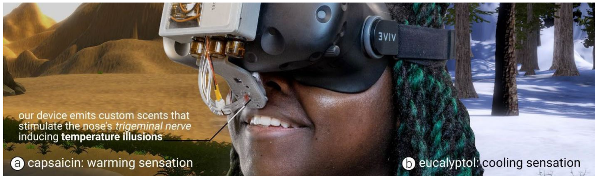
Figure 2: I engineered a thermal display that does not physically heat or cool but instead creates an illusion of temperature by stimulating the nose’s trigeminal nerve with different scents. This nerve detects temperature shifts but also chemicals like menthol or capsaicin, which are why breath mints feel cold and chilis feel hot. This work received a CHI 2020 Best Paper Award.
