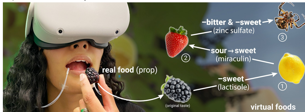
Figure 4: Taste retargeting selectively changes taste perception using taste modulators—chemicals that temporarily alter the response of taste receptors to foods and beverages. As our technique delivers modulators before eating or drinking, it is the first interactive method to selectively alter the basic tastes of real foods without obstructing eating or impacting the food’s consistency .
