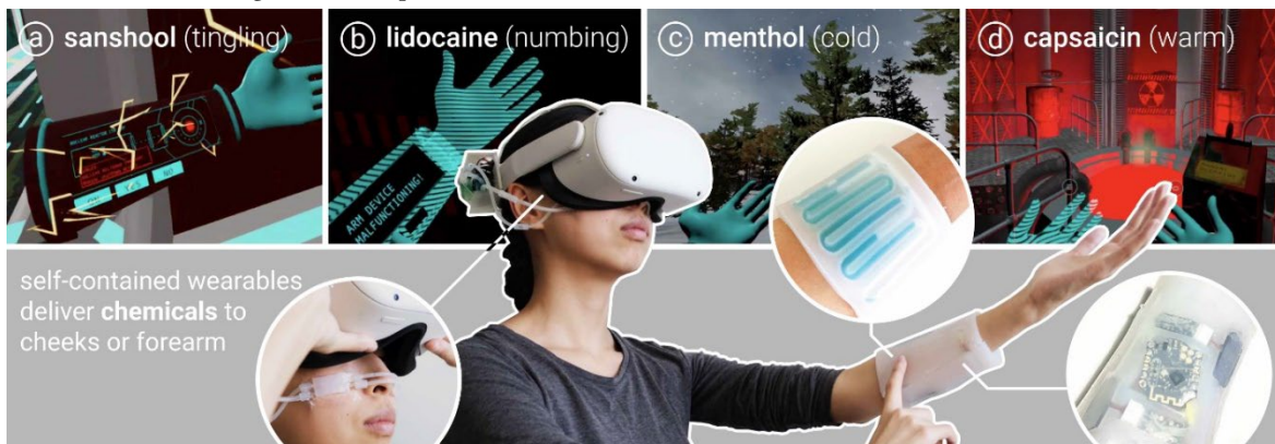
Figure 3: Chemical haptics leverages topical stimulants, chemicals that activate targeted skin receptors to render distinct haptic sensations. With one actuator, but different chemicals, the user can feel (a) tingling with sanshool, (b) numbing with lidocaine, (c) cooling with menthol, (d) warming with capsaicin, and even stinging with cinnamaldehyde.
