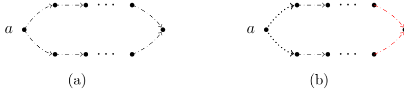
Figure 1.3: Dotted lines denote online queries. Solid lines denote offline queries. Dash-dotted lines can be either offline or online queries. Red lines denote ‘colliding’ queries.
