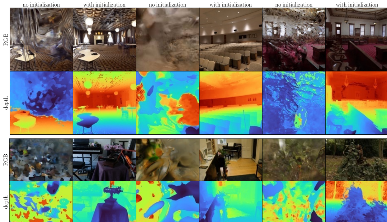
Figure 5.5: Image and depth maps produced by Nerfacto on the ballroom, auditorium, and courtroom scenes from Tanks and Temples at k = 25 , and the bonsai, room, and stump scenes from the Mip-NeRF 360 dataset at k = 10 . Not using high transmittance offset causes the optimization to get stuck with cloudy floaters.
