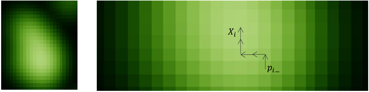
Figure 8 - result of \text{climb}[\text{climb}[\dots \text{climb}[p]]] . We assign a point p_i to its natural source when following the discrete gradient direction in the image. All points within this blob will belong to the same locus X_i
